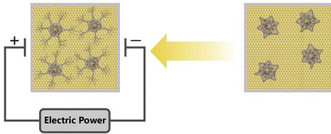
Fig. 3. Schematic of electrical stimulation of PC12 cells cultured on the gold nanoparticle-coated surfaces to neurite outgrowth.
