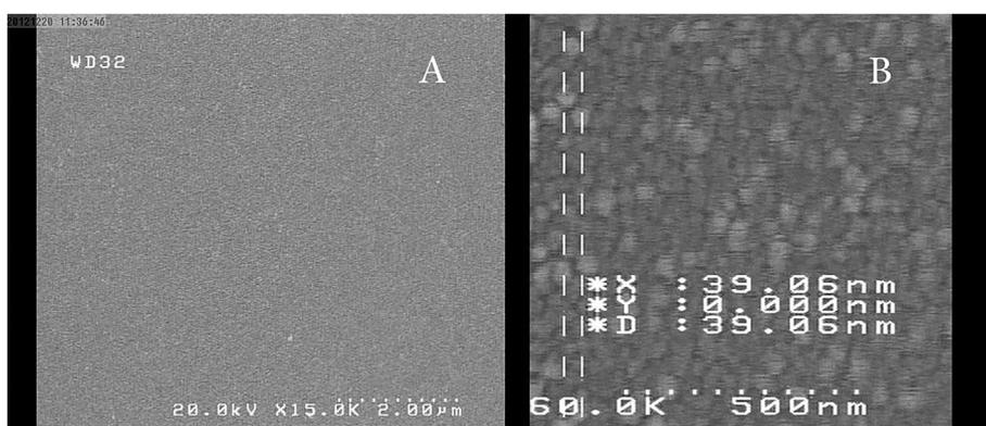
Fig. 1. FESEM images of the AuNP films on PEI-modified glass slide. (A) 15,000 $\times$  (B) 60,000 $\times$ .
